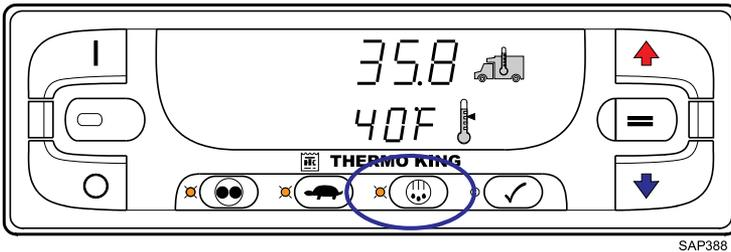
**Important:** During the defrost cycle, the box temperature will rise toward 50° F (10°C). This is normal and is caused by the defrost cycle warming the evaporator coil. Since the damper door is closed during the defrost cycle, this warm air is not allowed to pass into the truck box.
